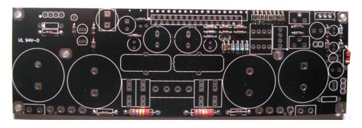
Here is how the board must appear after the first two steps. Take time to check if to each arrow on the figure above correspond to a resistor on the board, and if your board appears like the picture above. The colors of the resistors may be different, depending on the values chosen.
