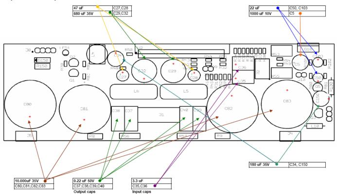
Pay attention to the polarity of each cap. A red "+" has been added to facilitate the identification of the polarity.
