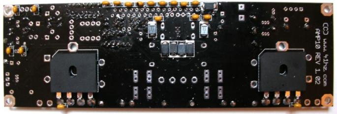
The seven diodes on the bottom are the only surface mount components, but are big enough not to worry. Pay attention to diodes direction: the thick line on the component MUST correspond to the thick line on the figure above. A diode soldered in the wrong direction may damage the amp irreversively.
