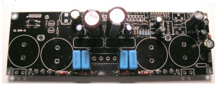
Check again the polarity of each cap comparing your board with the picture above. The positive pole's got a square soldering point. A reversed cap can explode and can cause injury. The four bulk caps can be soldered later, just before the power supply test. This way next step will be easier.
