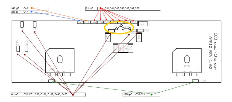
IMPORTANT: don't solder Capacitors C45 and C44. These must be soldered in the same holes of pin 4-8 and 9-12 of the TA2022. These caps will be soldered at the end, together with the TA2022.
