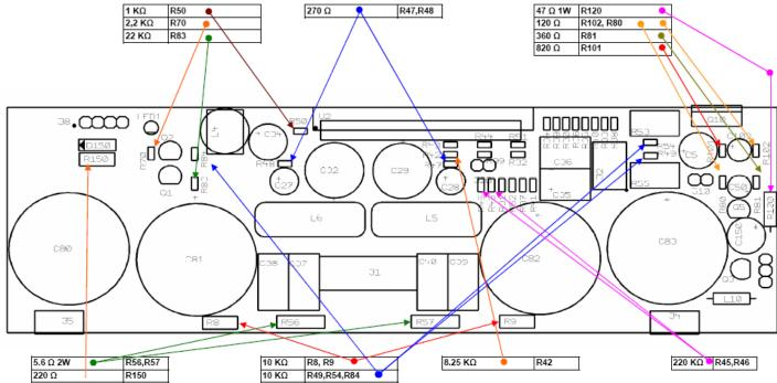
Other resistors are for on board power supply, on the right and under the bulk caps, for over/undercurrent and over/undervoltage sensing, for the on chip VN10 and for the external, optional relay.
