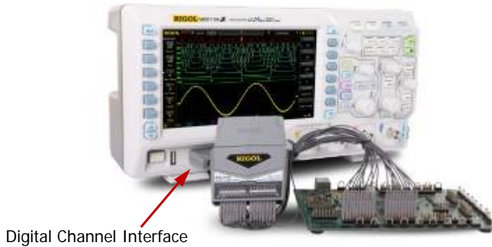
Figure 1-6 To Connect the Logic Probe
