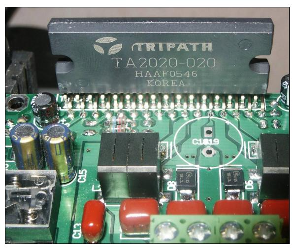
6. Last connect power connectors and you are ready for testing. For testing at low power no heat sink is required. For low to medium power applications the amplifier housing may be sufficient as a heat sink. For high power use like at full power into 4 ohm speakers, the amplifier can dissipate 20W of heat. Then, a 3 or 4°C/W heat
