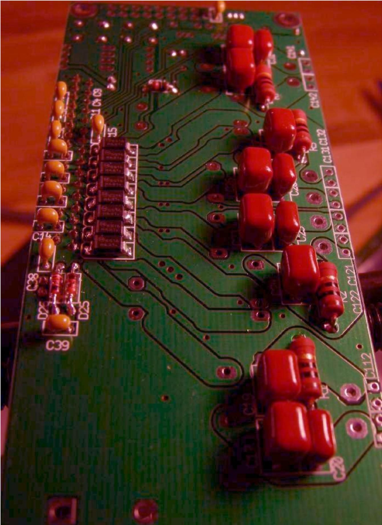
3. Turn the board over and continue by mounting 8 small diodes on the top side.
