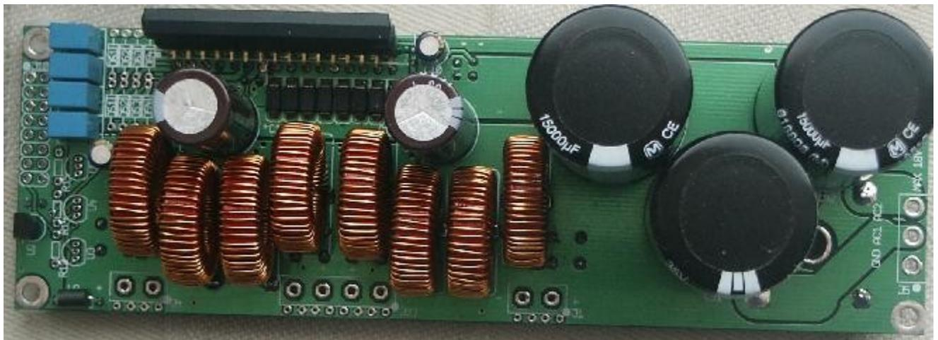
The two mounting holes on the power side of the PCB are connected to the ground plane, the two holes on the signal end of the board are not.
