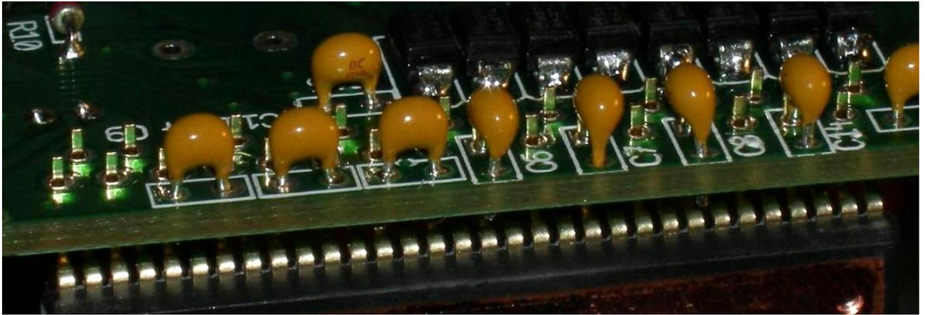
Solder the chip in place, making sure it is well aligned, horizontally and vertically.
