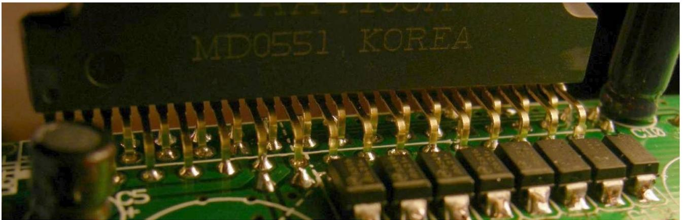
8. Continue with the two close-up bulk capacitors, C12 and C13. Again, note the polarity.
