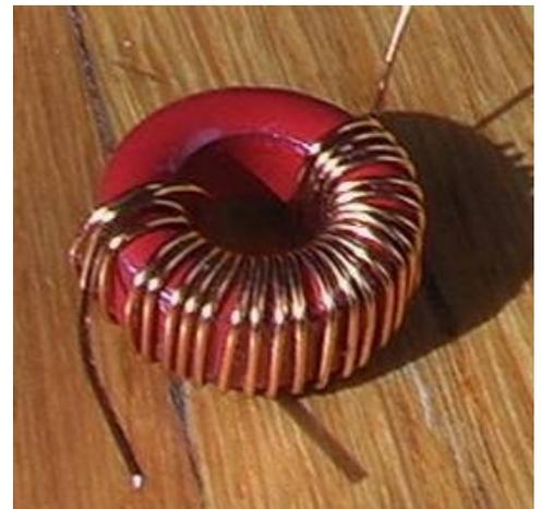
meter, measure the inductance. It should be 10 uH. If you do not have an inductance meter, count the turns.
